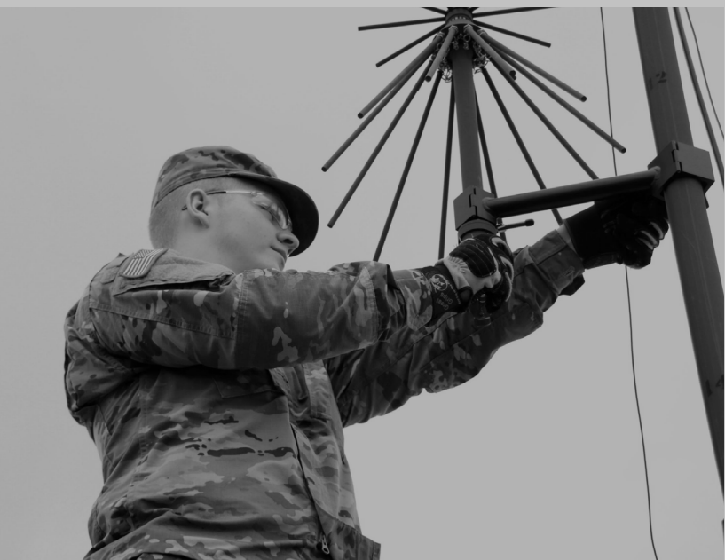
An air defense battle management system operator, 38 th Air Defense Artillery Brigade, assembles an omnidirectional, line of sight antenna. The antenna enabled communication with aviation assets during a unilateral joint training exercise that refined systems and concepts for enhanced tactical planning, coordination, and interoperability in a multidomain environment on Sagami General Depot, Sagamihara, Japan, September 17, 2019. (Photo by SGT Raquel Birk)
