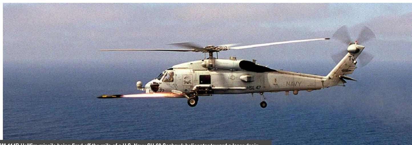
An AGM-114B Hellfire missile being fired off the rails of a U.S. Navy SH-60 Seahawk helicopter toward a laser designated surface target during training off the coast of San Clemente Island, CA, on August 25, 1999. (DoD photo by Petty Officer 1st Class Spike Call, U.S. Navy.)
