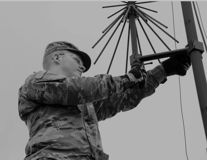
An air defense battle management system operator, 38<sup>th</sup> Air Defense Artillery Brigade, assembles an omnidirectional, line of sight antenna. The antenna enabled communication with aviation assets during a unilateral joint training exercise that refined systems and concepts for enhanced tactical planning, coordination, and interoperability in a multidomain environment on Sagami General Depot, Sagamihara, Japan, September 17, 2019. (Photo by SGT Raquel Birk)
