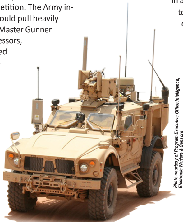
The Tactical Intelligence Targeting Access Node's (TITAN) modular systems mounted on a Joint Light Tactical Vehicle contribute to its deep sensing intelligence gathering capabilities.
