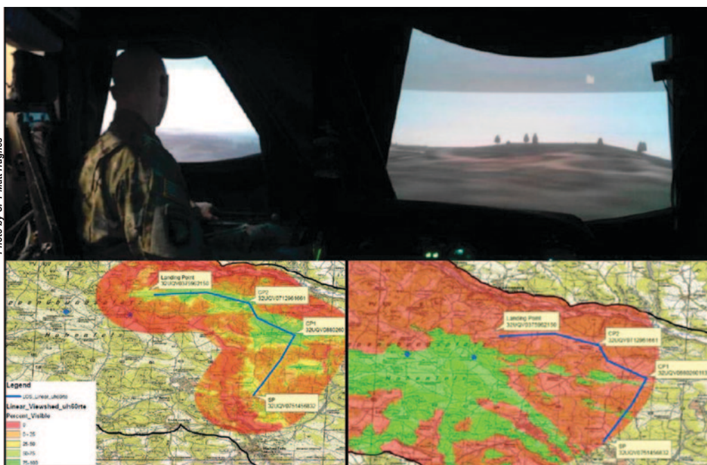
(Clockwise) In November 2015, CW2 Deuel flew the UH-60 flight simulator at Illersheim, Germany along a route he templated for HTA, Germany using SAGE. He modeled air ambush teams' radial line-of-sight and generated a linear viewshed along his flight path to determine visual detection probability along the route.
